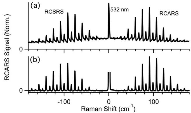
Fig. 2. Spectra (corrected for dark counts) from 5% N<sub>2</sub> in Ar at 294 K and 1 bar for delays of (a) 0 ps and (b) 200 ps.
