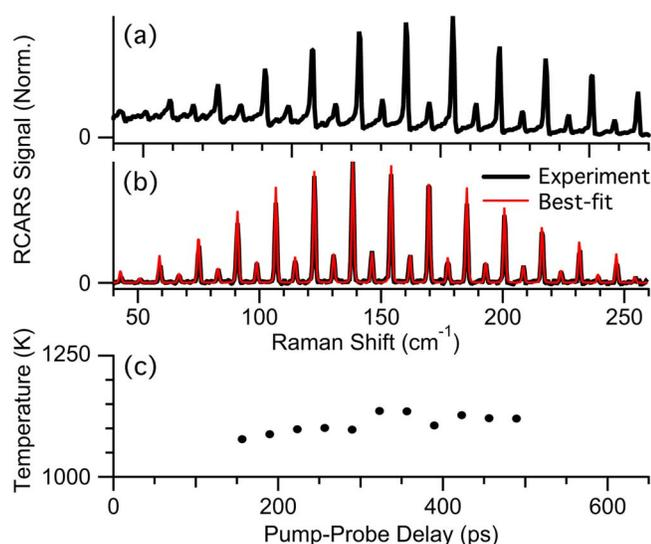
Fig. 4. (Color online) Spectra obtained on the fuel-rich side of a  $CH_4$  flame for delays of (a) 0 ps and (b) 260 ps. (c) Evaluated temperatures as a function of delay.
