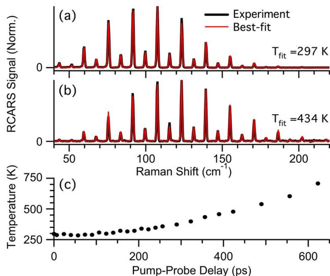
Fig. 3. (Color online) Fitted experimental spectra from  $N_2$  at 294 K and 1 bar for delays of (a) 0 ps and (b) 360 ps. (c) Evaluated temperatures as a function of delay.
