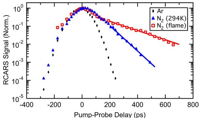
Fig. 1. (Color online) Spectrally integrated RCARS signal plotted as a function of the pump-probe delay.
