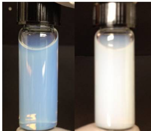
Figure 2. Pictures of the expanded particles at room temperature (left), and the collapsed particles at \sim 45^\circ\text{C} (right).
