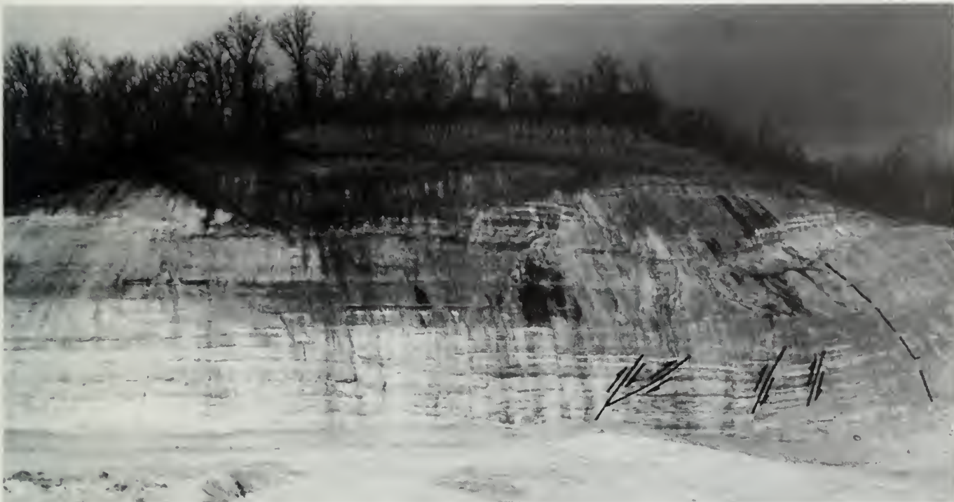
Figure 17 West wall of the north pit at the Lone Star mine shows loess on top of the ridge and several small faults in the Clear Creek Chert. The distance from the top of the ridge to the pit floor is 161 feet (49 m). The black patches are dead vegetation. The location of the described section (fig. 25) is shown by a dashed line. Photo by J. M. Dexter, ISGS.
