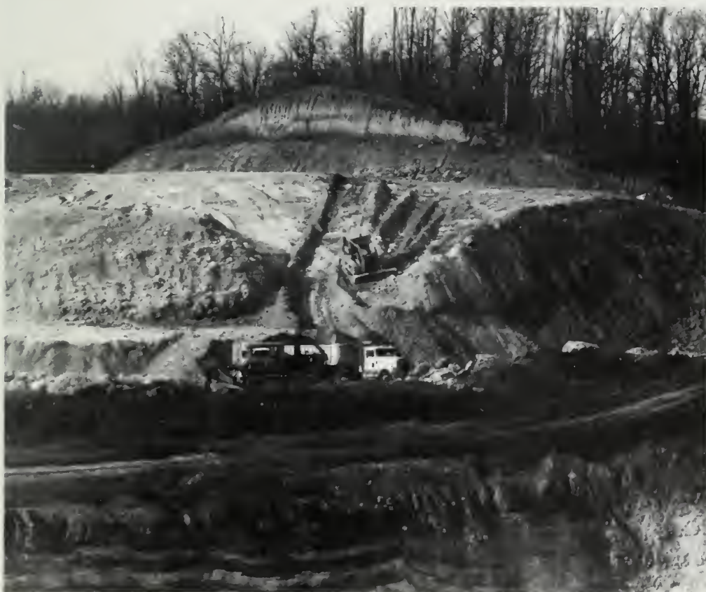
Figure 15 West wall of the south pit at the Lone Star mine in the Clear Creek Chert (site 65, appendix A and plate 1). The photo shows where loess and massive chert beds have been stripped to expose the microcrystalline silica. The silica is mined for use in portland cement. Photo by J. M. Dexter, ISGS.
