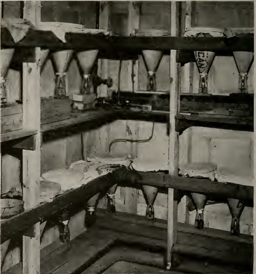
Fig. 6.—Funnels in position on rack. In this assembly, each funnel rests inside a double ring of copper tubing (as on funnel at extreme lower left) through which flows live steam. The steam produces the heat that dries out the sample and drives the animals out of it. Cotton or a small rag is tamped between the end of the funnel and the bottle of preservative to prevent escape of specimens.
