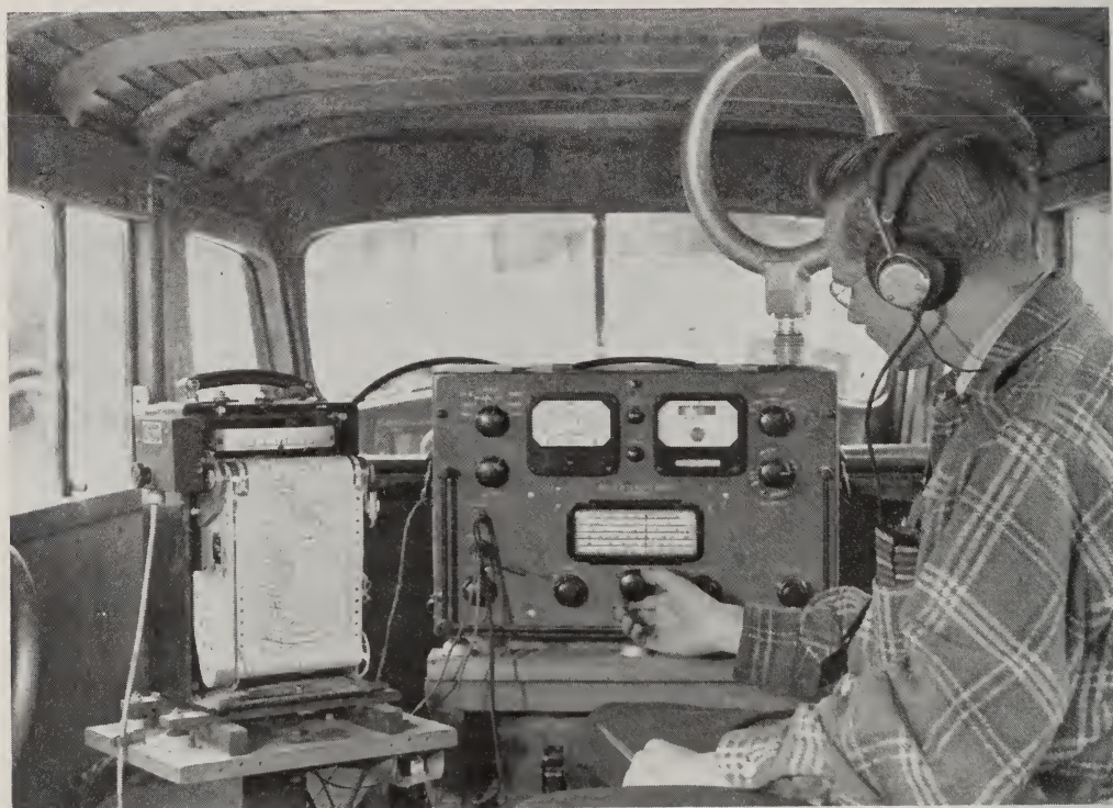
FIG. 4.—Operator in working position. The 308-B field intensity meter (center); Esterline-Angus recorder and Clark speedometer drive (left).
