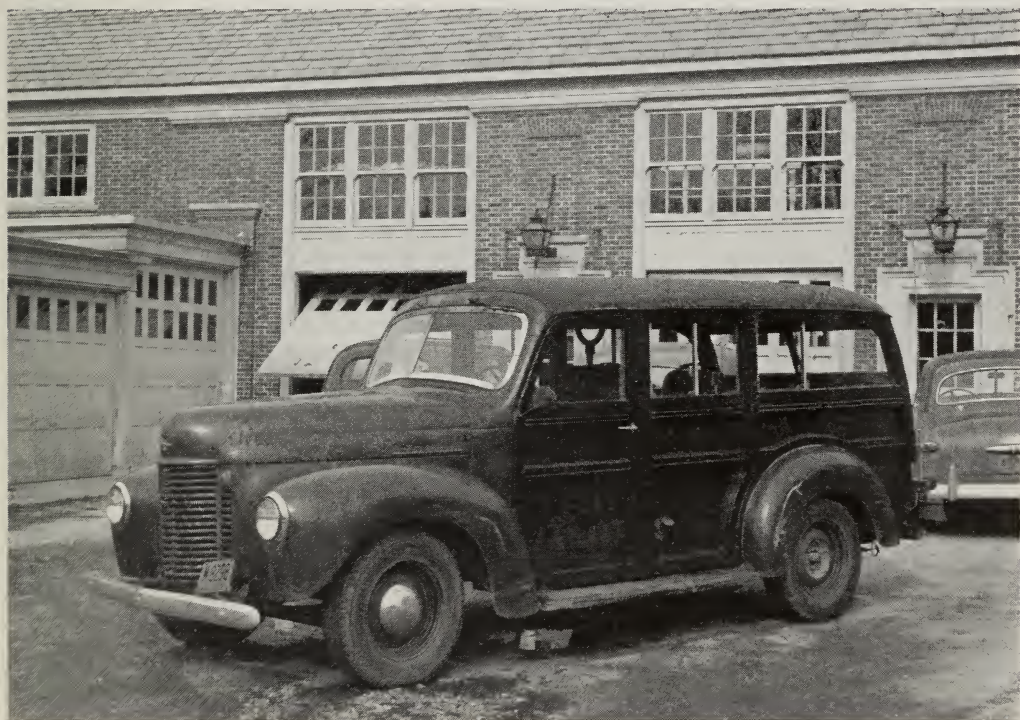
FIG. 3.—Wooden-bodied station wagon with permanently mounted radio field intensity measuring equipment.
