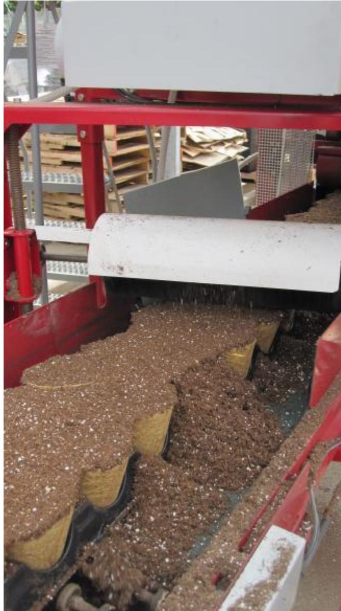
Fig. A.1. As trays of straw pots exit the gravity-fed filling machine (model PM1100, Agrinomix, Oberlin, OH) a rotating brush sweeps off excess potting mix. Proper adjustment of this brush was critical in the prevention of container damage and tipping.
