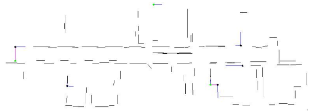
Fig. 2. The SLAM module creates a metric line map representing walls and other straight surfaces in the environment.
