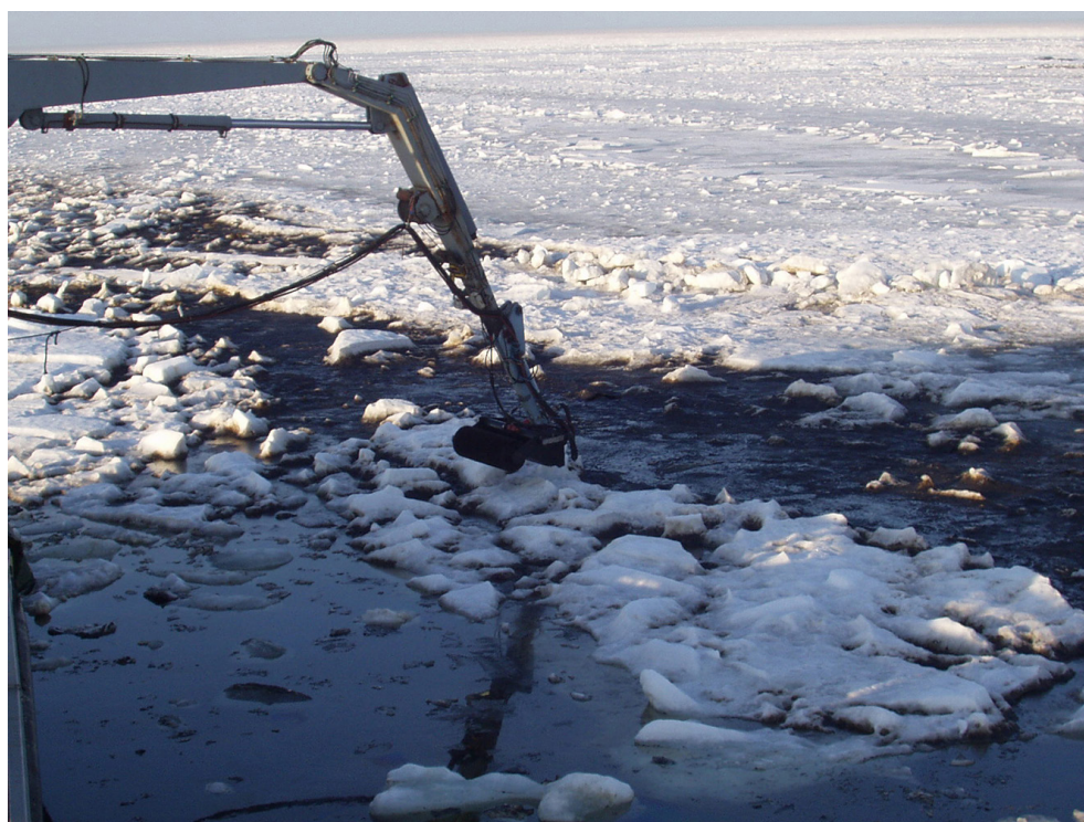
Oil being cleaned from ice (Photo: Jouko Pirttijärvi/SYKE).
