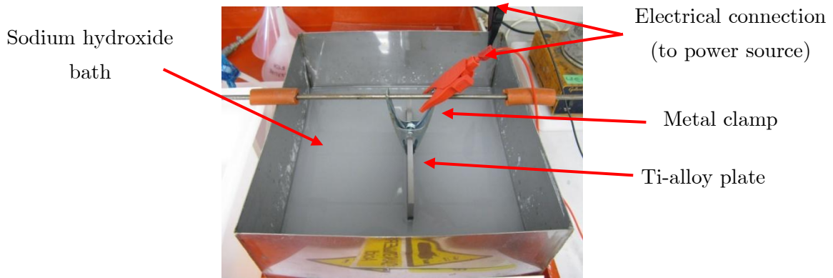
Figure 4.7. Ti-alloy plate in sodium hydroxide bath during anodising.
