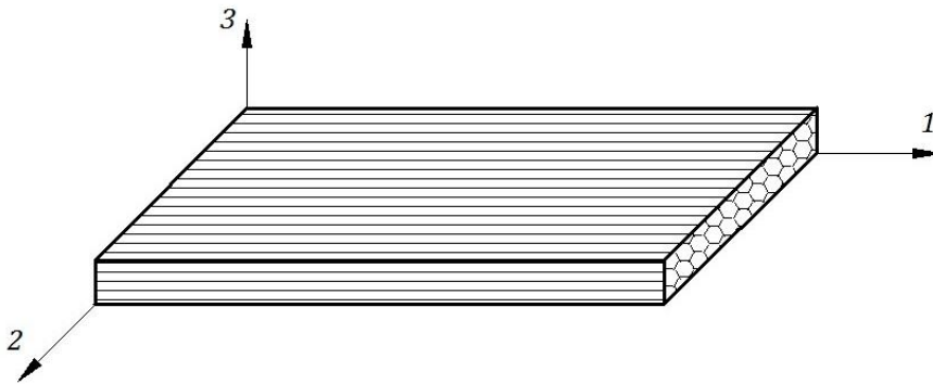
Figure 4.3. Directions considered for the mechanical properties of the CFRP laminates.
