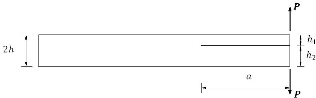
Figure D.1. Schematic representation of the ADCB test specimen (width, B ).
