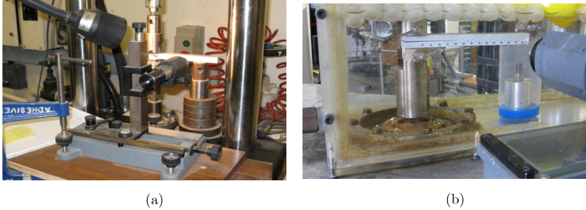
Figure 4.21. Set-up used in the mode I fatigue in (a) “dry” and (b) “wet” conditions (polypropylene spheres in the tank to minimize water evaporation).
