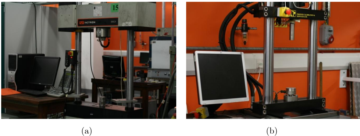
Figure 4.19. Servo-hydraulic testing systems employed in the fracture mechanics mode I fatigue tests: (a) INSTRON 8501 and (b) Phoenix.
