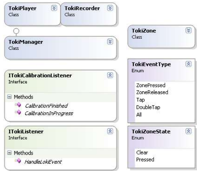
Figure 6: Main components of the Toki API.
