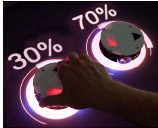
Figure 5. A user rotates a tangible to adjust the percent value. Physical/digital conflicts are avoided by rotating the other tangible, thereby preventing the total from exceeding 100%
