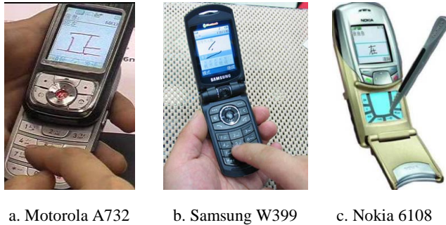
Fig. 1. Phones supporting handwriting recognition with touch-sensitive keypad, which are evaluated in the study
