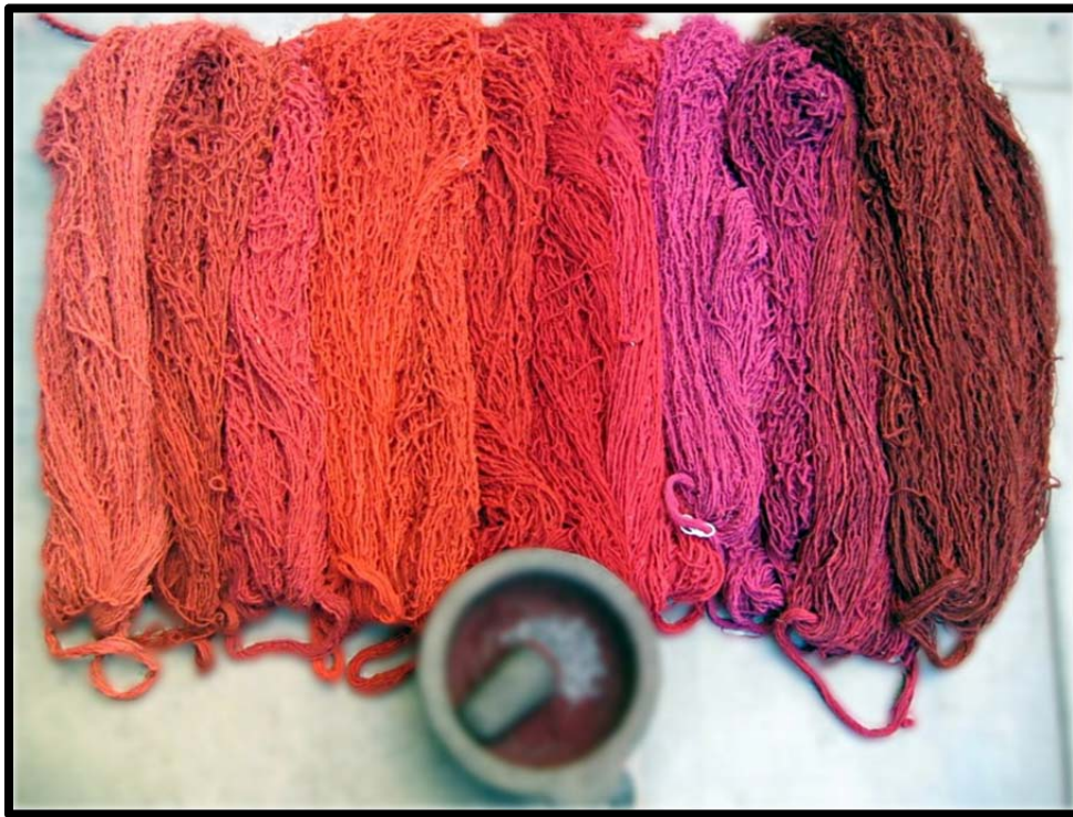
Figure 1. Wool samples dyed with cochineal with different mordents and pH. Image by Eric Chávez.
