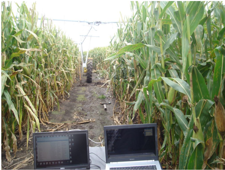
Figure 3.14: Temporary testbed for UG2AG and AG2UG experiments inside a crop area.
