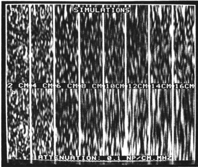
Figure 8: Simulated B-mode scans (after gray level normalization) of a cloud of scatterers in a medium without attenuation (a) and a medium with attenuation 0.1 Np/cm.MHz (b), at several distances to the transducer. The dimensions are the same as in figure 5.
