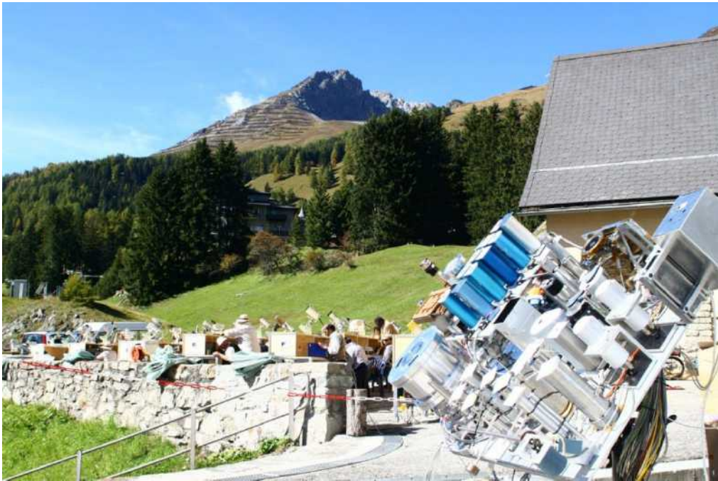
Figure 1 Radiometers of the World Standard Group on a solar tracker, together with other Solar Irradiance instruments (picture courtesy of PMOD/WRC, Davos)
