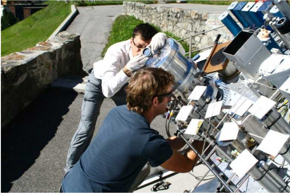
Figure 87 Initial alignment of CSAR to the Sun. The picture shows the author with a beam splitter, and André Fehlmann (PMOD/WRC) adjusting the tilt of CSAR.
