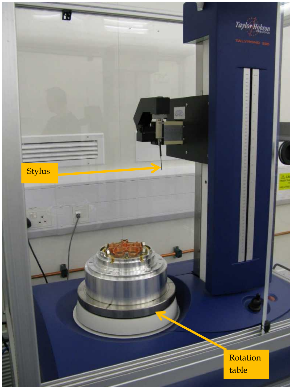
Figure 82 Measurement of alignment of detector stage to outer support structure
