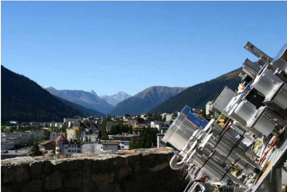
Figure 139 CSAR on the solar tracker with World Standard Group instruments.
