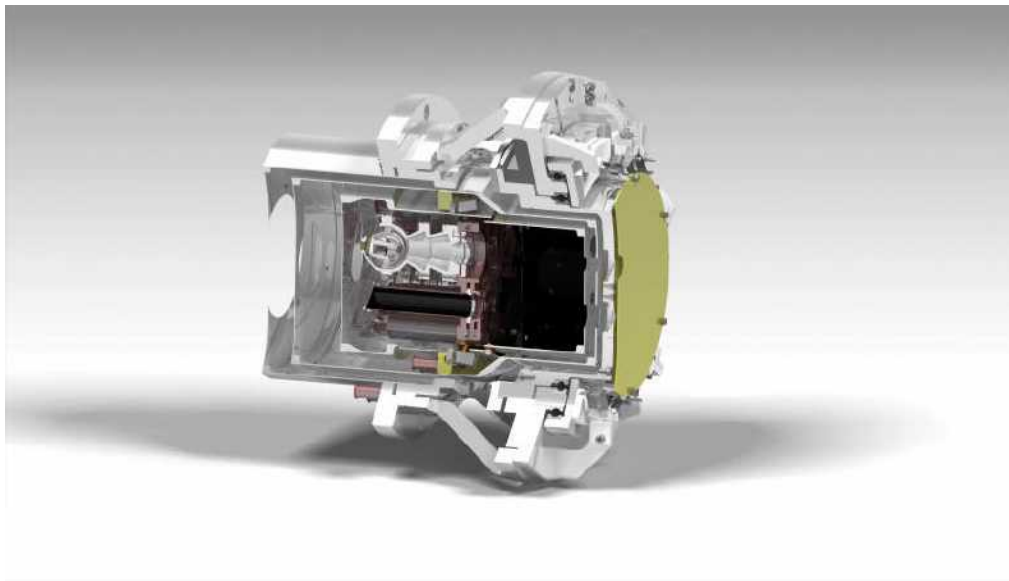
Figure 37 CSAR radiometer head - 3D model, cross section
