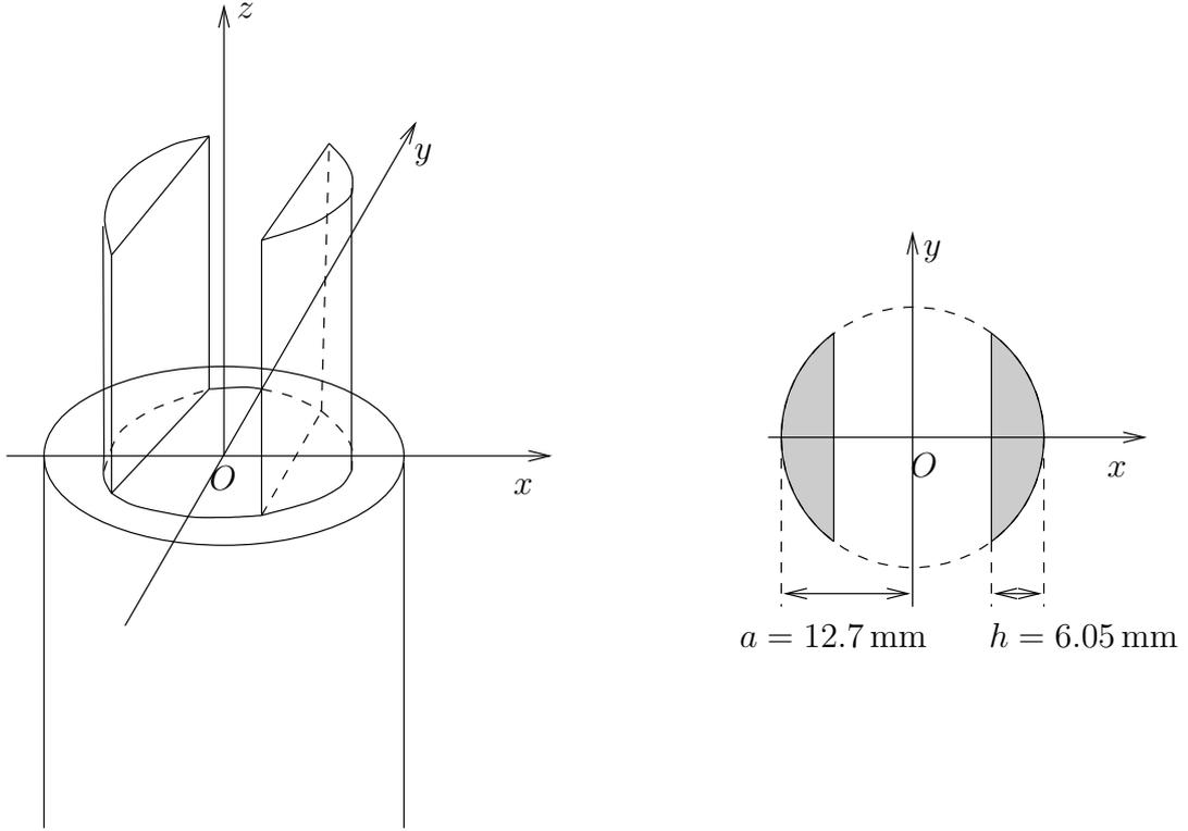
Figure 1: Diagram of tuning fork densitometer.
