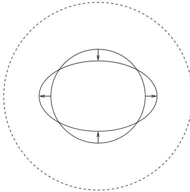
Figure 6: Quadrupole-style imposed motion on surface of cylinder.
