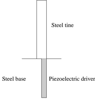
Figure 3: Diagram of forcing mechanism.
