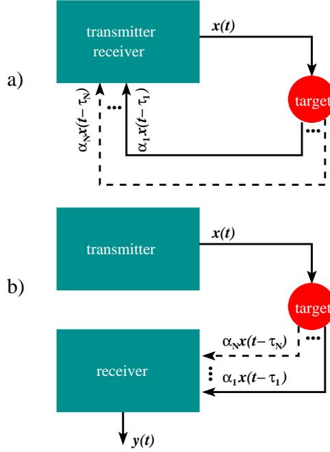
Figure 1: Two schemes for inducing bifurcations in a receiving system: (a) direct feedback scheme and (b) parallel systems.
