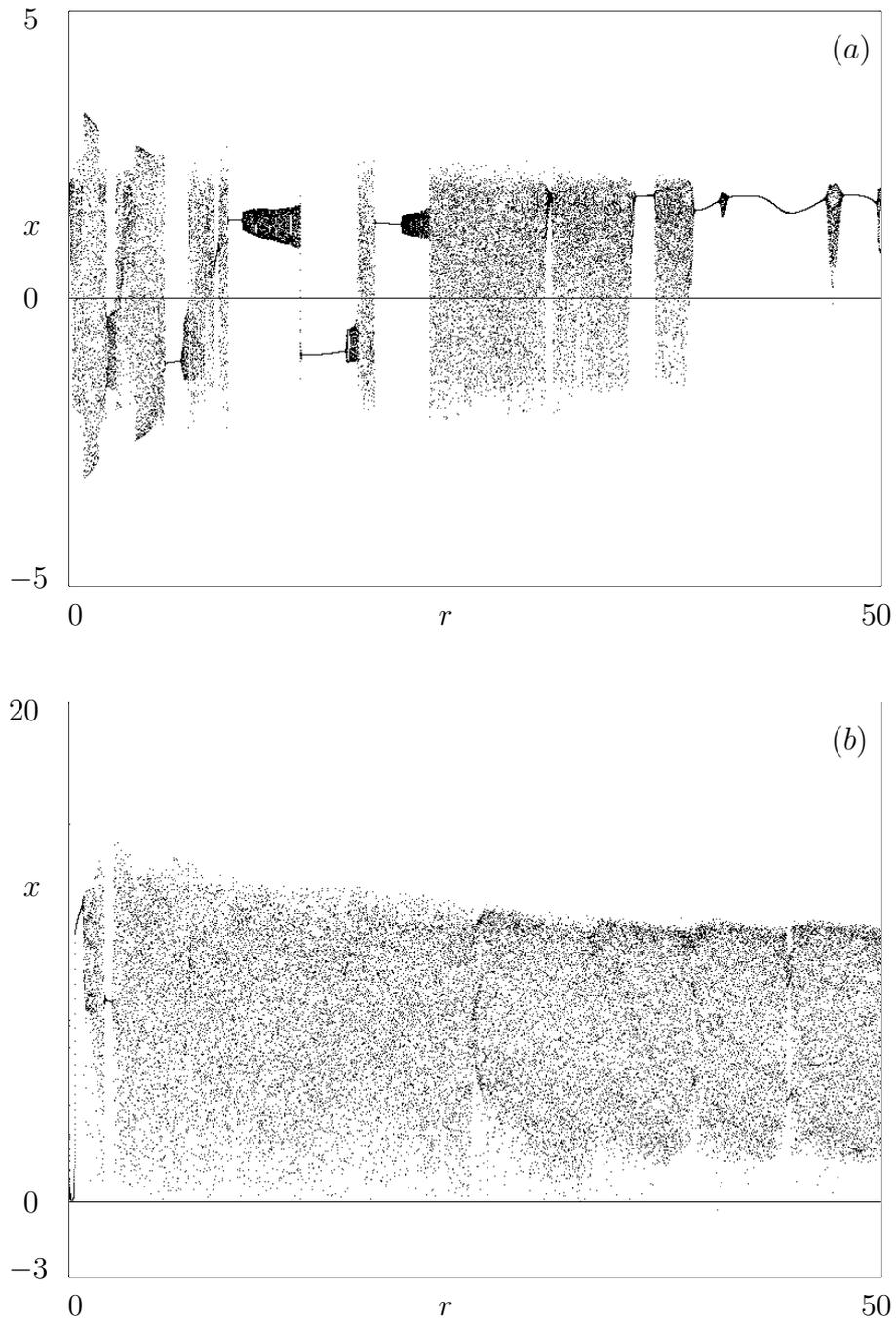
Figure 3: Examples of bifurcation diagrams for (a) a forced Duffing oscillator with parameters  $c_1 = 0.04$ ,  $c_2 = 1$ ,  $F = 0.3$  using a stroboscopic Poincaré section with  $t = 2\pi n + \text{const}$  and (b) the Rössler system with parameters  $a = 0.2$ ,  $b = 6.5$  using a Poincaré section with  $y(t) = 0$ . Parameters  $\alpha_{0,1,2}$  and  $\tau_{0,1,2}$  were defined for  $c = 1$ ,  $D = 10$ , and  $d = 8$ .
