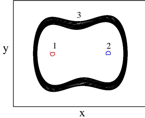
Figure 4: Multistability in a forced Duffing oscillator with delayed feedback for parameters values  $c_1 = 0.24$ ,  $c_2 = 1$ ,  $F = 0.27$ ,  $r = 2$ ,  $D = 10$ ,  $d = 8$ .
