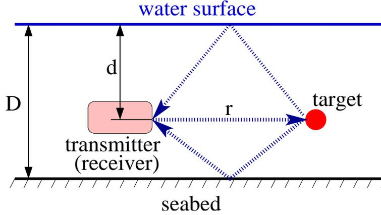
Figure 2: Geometry of two-path signal propagation.
