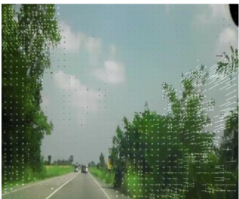
Fig. 3. Motion vectors in a sample scene when the car moves along the road.
