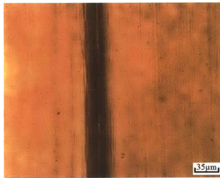
Figure 4-14: Microscopic image of scoreline with w = 69.8\mu\text{m} , d_s = 34.9\mu\text{m} .
