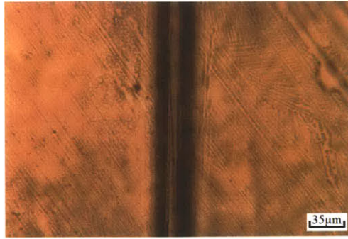
Figure 4-15: Microscopic image of scoreline with w = 33.3\mu\text{m} , d_s = 16.7\mu\text{m} .
