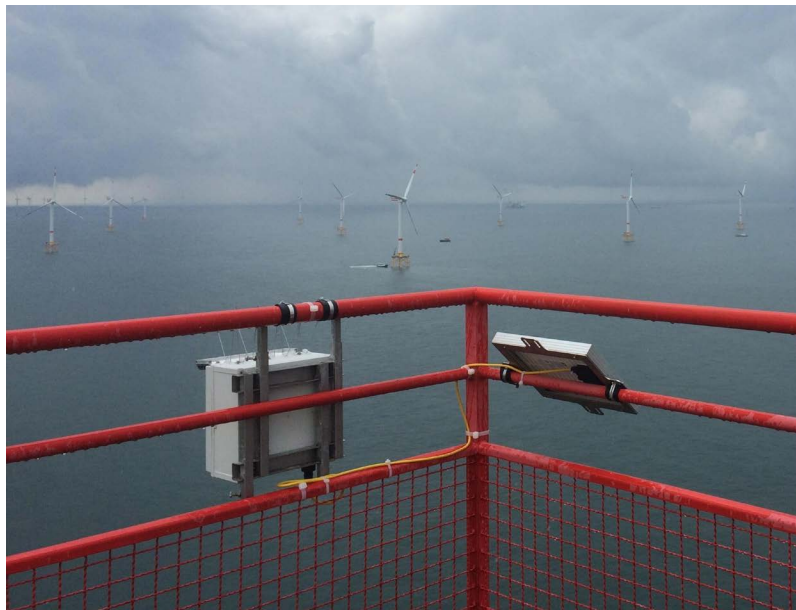
Figure 2. Batcorder installed on the helicopter winching platform at the back of the nacelle of turbine I1.
