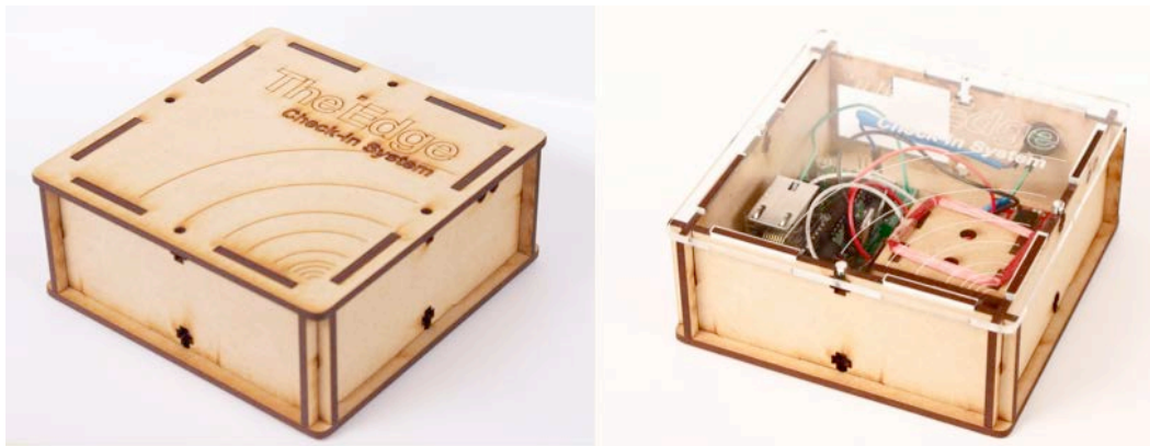
Figure 42: A networked thermal printer prints a personal user profile ticket with their skills, interest and workspace location for each user that has checked-in by touching a checkin-point (bottom pictures) with their library user card. The design is based on open source hardware and software ( http://arduino.cc ), and digital fabrication methods such as CAD and laser cutting.
