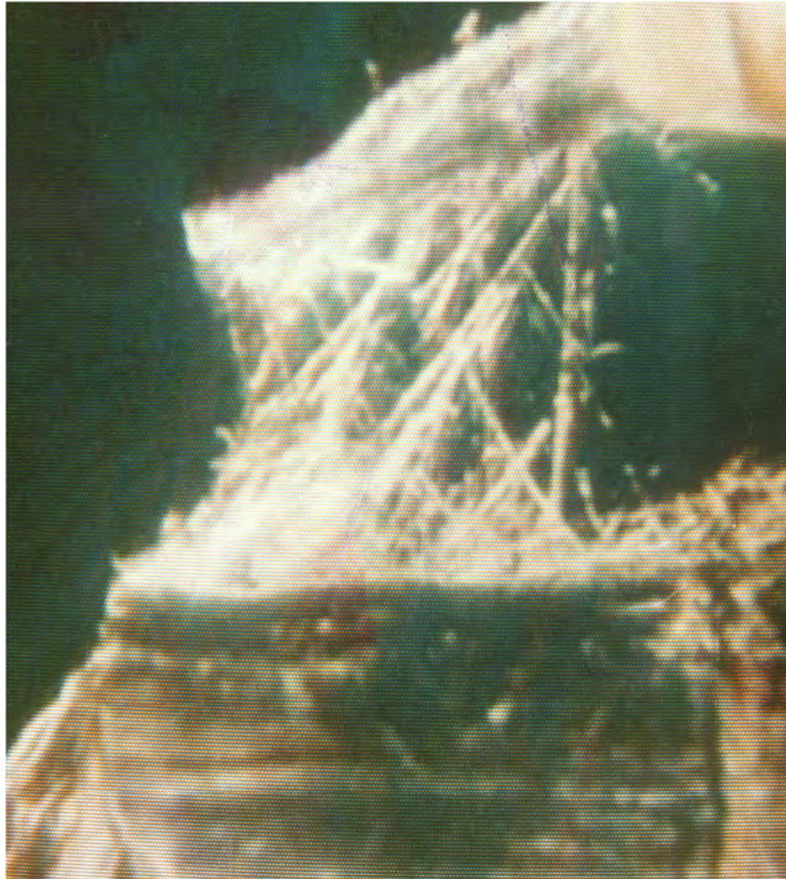
Figure 36: Blue asbestos fibre. Photo courtesy Peter Gordon.
