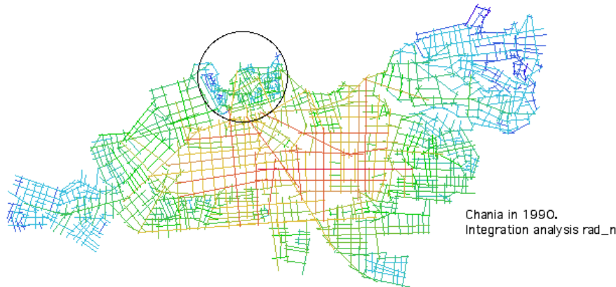
Fig. 23 Integration analysis rad_n of Chania in 1990. The circle indicates the red dots in scattegrams in Fig. 15 and Fig. 16
