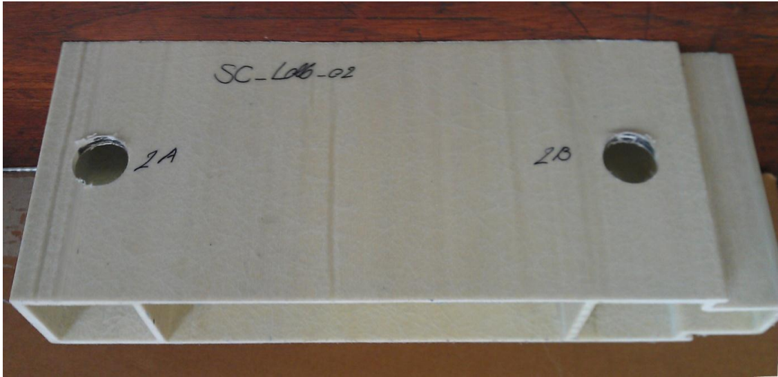
Figure 3. Bearing mode of failure of stud-column section in specimens WU-sc-Ldb-2A and WU-sc-Ldb-2B.
