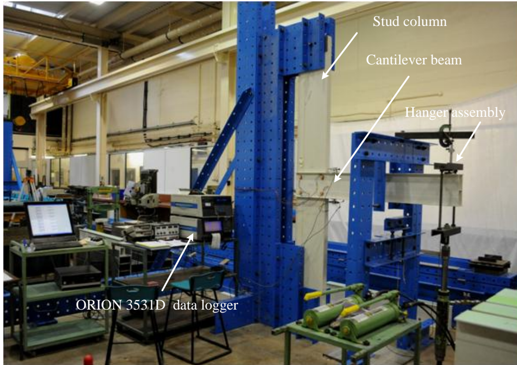
Figure 6.23. Test rig with attached ORION 3531D data logger, the computer, hanger assembly, load cell and instrumented specimen.
