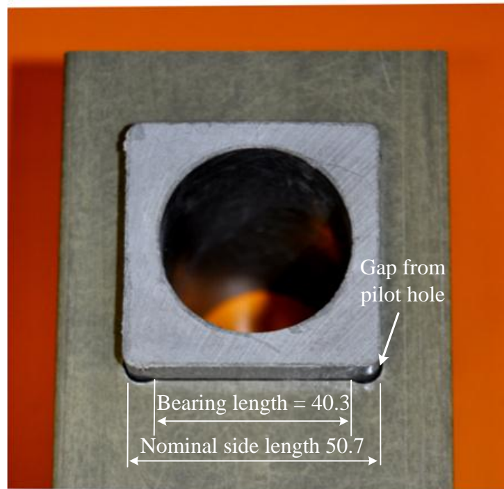
Figure 5.11. Bearing length in millimetre in square notch with presence of drill pilot holes at the corners of the rectangular shape.
