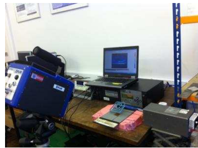
Figure 14. The photo of PEC thermography set-up
