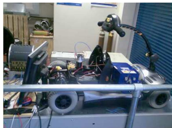
Figure.5. University of Glamorgan Hydrogen Scooter vehicle test-bed (Thanapalan et al , 2008)
