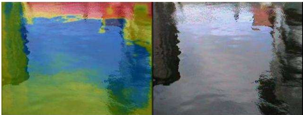
Figure 4: Thermal and digital image for a deeply submerged discharge
