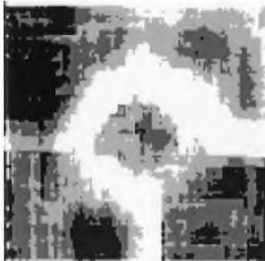
Figure 3.19: Segmentation of texture montage by fractal signature method using 17 \times 17 estimation boxes
