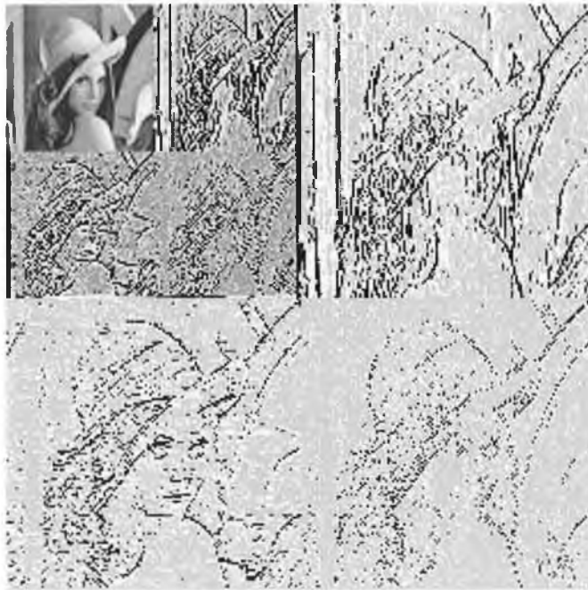
Figure 4.1: Two stages of wavelet decomposition of Lena
