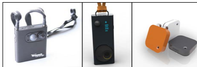
Figure 1. Wearable cameras: SenseCam (left; http://research.microsoft.com/ ), Autographer (middle; www.autographer.com/ ) and Memoto (right; http://memoto.com/ ).
