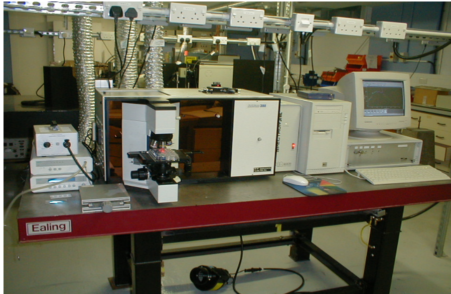
Figure 124: LabRam Raman spectrometer at the University of Greenwich used to conduct Raman experiments.
