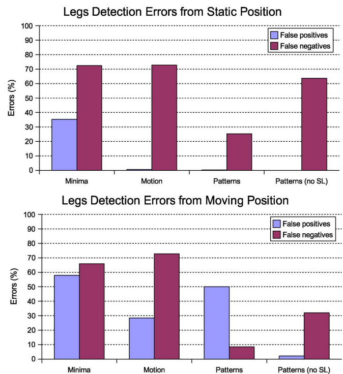
Fig. 14. Comparison of leg-detection errors using algorithms based on distance minima, motion detection, and leg patterns (with and without SL). Errors are expressed as ratios of false positives versus total leg detections and as false negatives versus total detectable persons.
