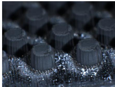
Figure 3.2: Image of some of the MWNT fins in a staggered array
