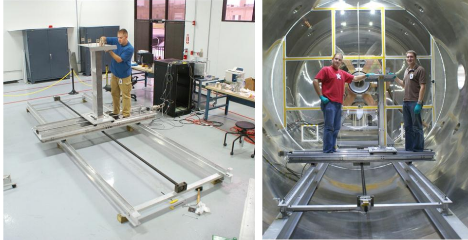
Figure 3.10: (left) Two-axis translation stage during construction. The range of travel is 2.5 m in the Y direction and 5 m in the Z direction. Each axis is ballscrew driven controlled by high precision step motors and limited by inductive limit switches. Leading edges are covered by grafoil™ to limit sputtering from the aluminum frame. (right) Translation stage shown installed in the exhaust region of the vacuum chamber looking upstream.
