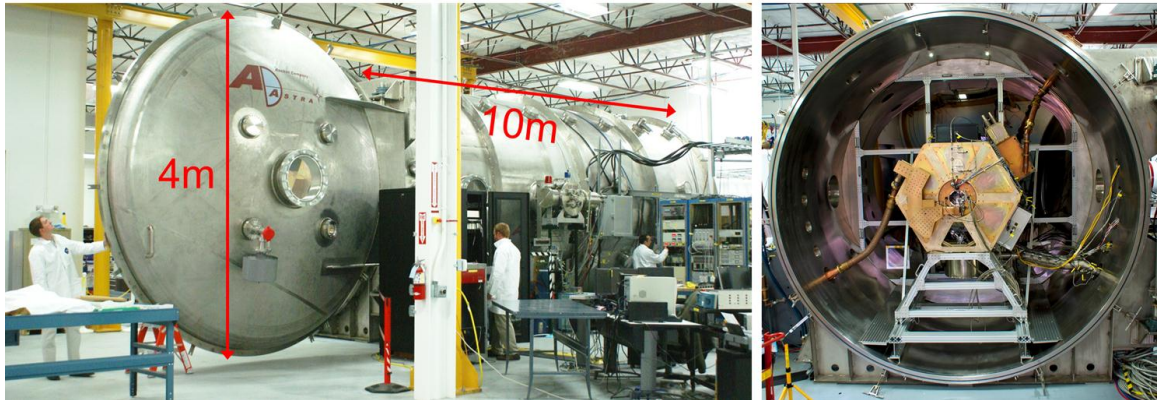
Figure 3.8: (left) Preparing the experiment at the 150 m 3 vacuum facility located at the Ad Astra Rocket Company. (right) The VX-200 Plasma source mounted coaxially to the chamber in the front end of the chamber. Copper coaxial RF transmission lines are fed from either side into RF matching networks for each stage of the rocket. Onboard sensors, data, and pressurized helium (for cooling the superconductor) are fed out to the right.
