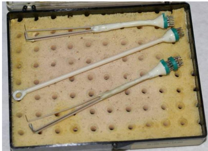
Figure 4.19: Probes designed to measure high frequency plasma phenomena. The top and bottom probes are identical in design featuring two tungsten electrodes spaced \sim 12 mm apart with a small B-dot coil in between. An individual B-dot probe is shown in the middle, but was not used in this experiment. The power spectrum is measured between the two electrodes.
