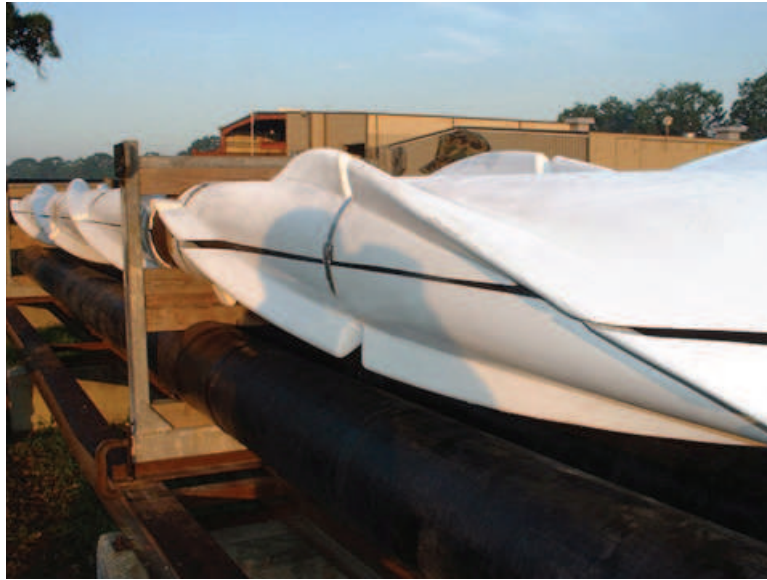
Figure 1.7 : Actual Strake for Risers (Courtesy: VIVsolutions.com)
