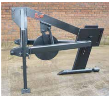
Figure 6: Mole plough showing foot and expander
