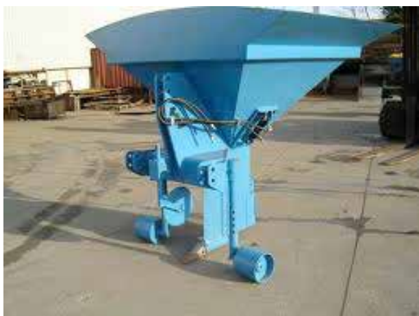
Figure 7. Gravel mole plough showing hopper
