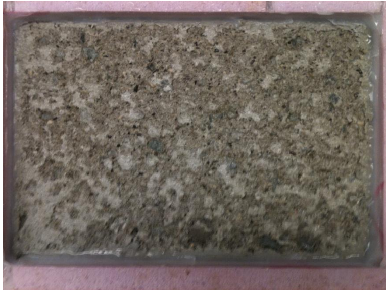
Figure 3. ASTM C672 exposure for Mix #13 (50%LA 50%SG120 0.42w/c) at 25 cycles where coarser sized pieces of scale were observed
