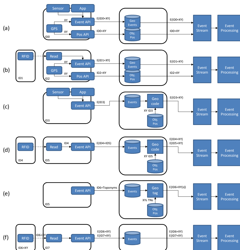
Figure 4.3 Methods to geo-enable events (Source: Erik van der Zee, 2013.) Note: For RFID also Bluetooth, NFC, or similar methods can be read.
