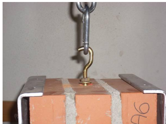
Figure 2: Failure by splitting of anchor head.
