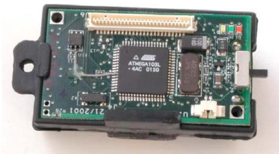
**Figure 1: Berkley Micra2 Wireless Sensor Mote**
