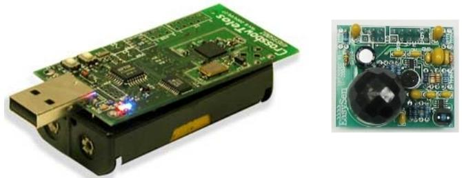
Figure 4. Crossbow telosb mote and EasySen sensor board
