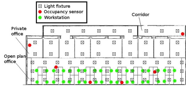
Figure 3. Office plan including occupancy sensor and workstation placement
