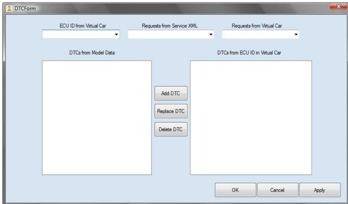
Picture 4.2 –DTC form used by the end-user to edit DTCs.
