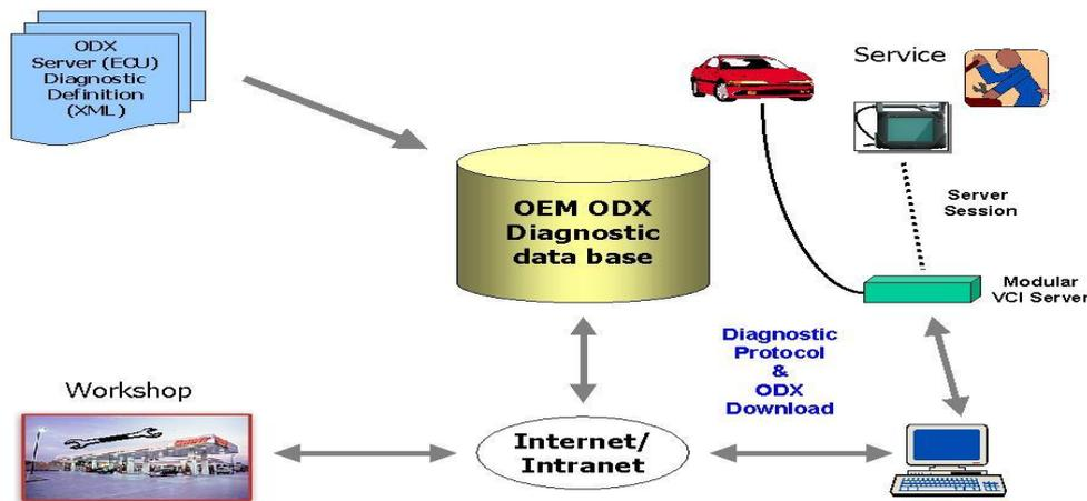
**Figure 2.0 – ODX central source diagnostic data process.**
