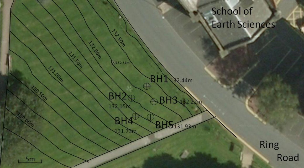
Figure 3.7: Test site at the University of Birmingham with elevations of the borehole covers of BH1, BH2, BH3, BH4, and BH5, with topographic lines of interpolated elevations of the surrounding area of the test site (taken out of a map of the Estates Services of the University of Birmingham, 2001; satellite image © Google Maps).
