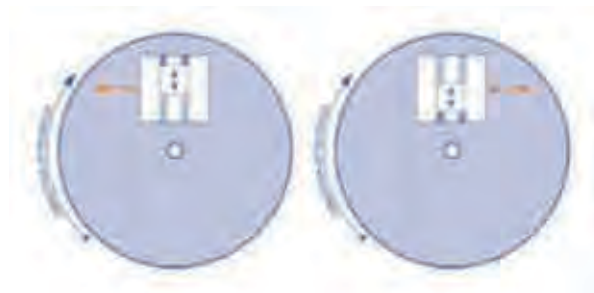
FIGURE 2.8: Gyroscope. Rotation forces the mass to move toward the outer edge when moving in the clockwise direction and moves towards the inner edge when moving in the anti-clockwise direction.
