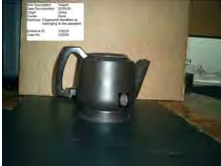
FIGURE 4.4: Upon successful recognition the user is presented with contextual information specific to the object
