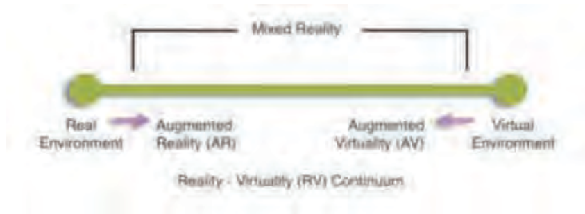
FIGURE 2.1: A Simplified Representation of the RV Continuum. Reproduced from Milgram et al. [21]
