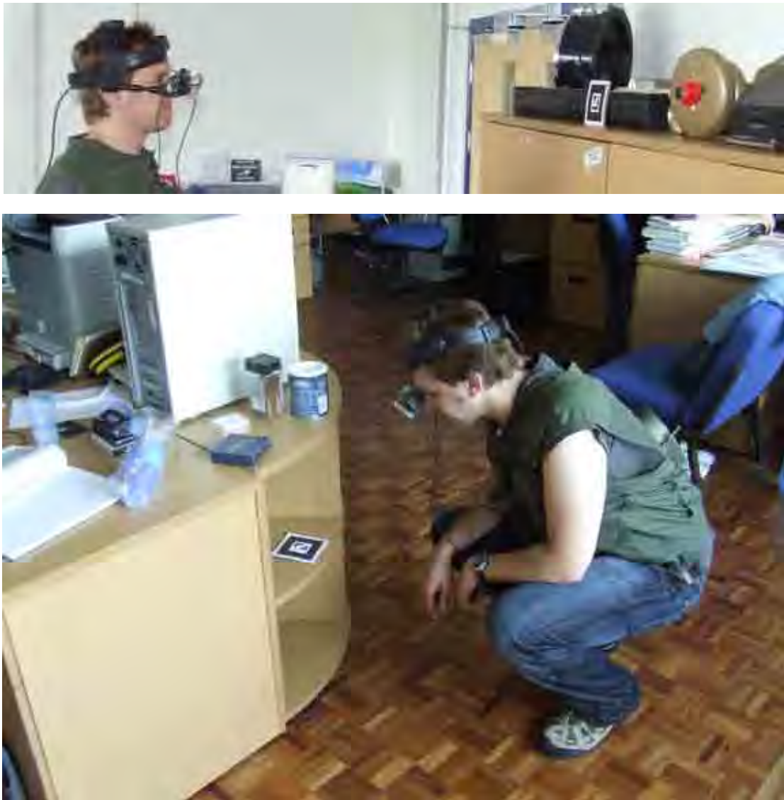
FIGURE 7.6: User Trial - X^4 wearable computer fitted into vest for non-invasive mobility.
