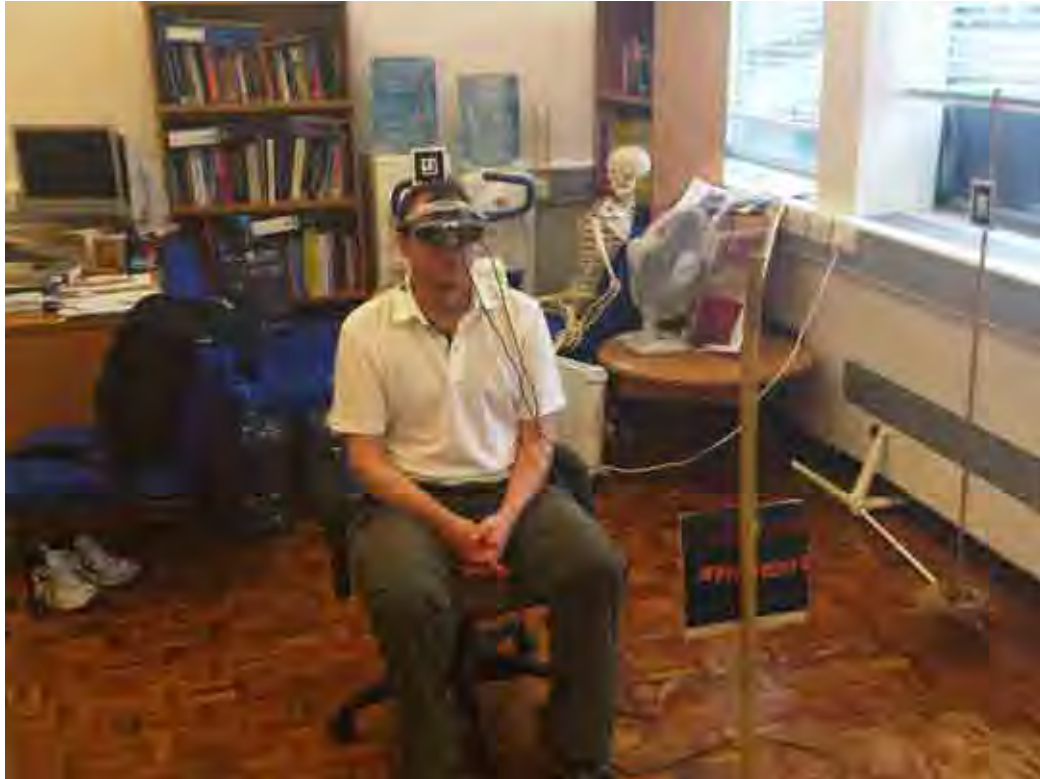
FIGURE 5.13: User Surrounded by 4 markers at per compass intervals, each marker displays a randomised block of three items.
