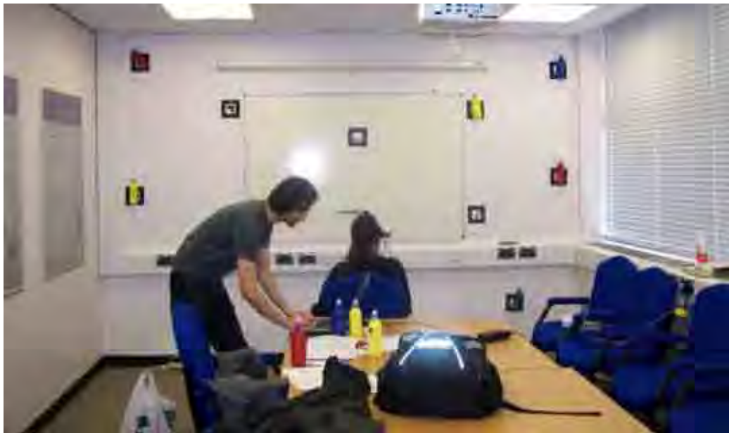
FIGURE 6.5: Real World Experiment Scene - figure demonstrates real bottles placed over markers, in the AR condition synthetic equivalents are presented in place of the marker.
