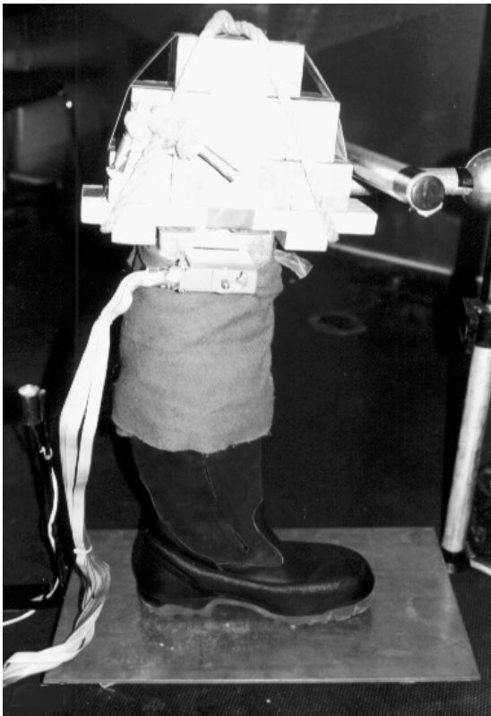
Figure 3. Setup for insulation measurements with thermal foot model.
