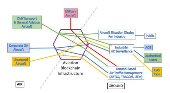
Figure 1. Notional design of blockchain-mitigated channels of communication. Chaincode (aka 'Smart Contracts') routes the information appropriately between aircraft and the ground-based ATM and other support services.
