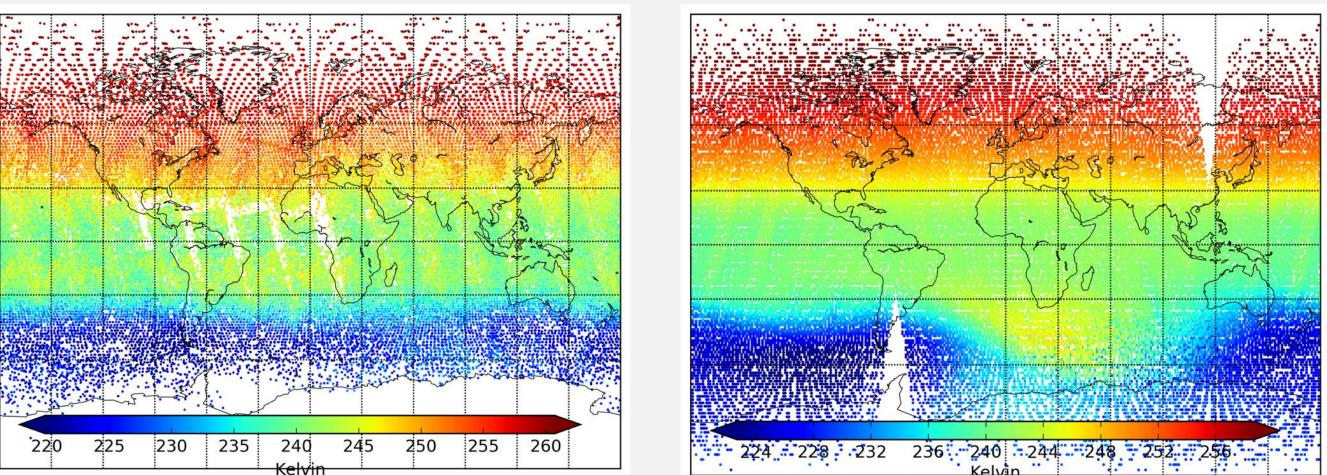
Real (left) vs. simulated (right) MISTiC observations (Channel 2359.77 cm-1). Difference between the real and simulated data is due to the non local-thermal equilibrium (NLTE).
