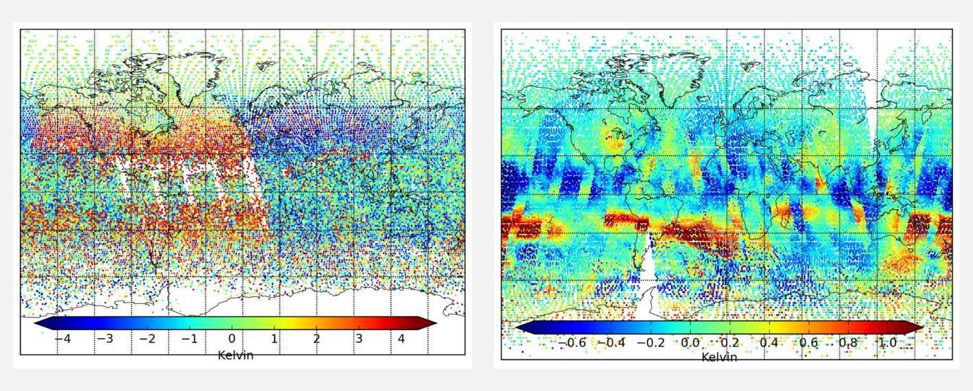
The OMF statistics for the MISTiC Chan. 2359.77 cm<sup>-1</sup>) (left: real and right: synthetic OSSE observations). The large difference between the real and OSSE statistics is due to the NLTE.
