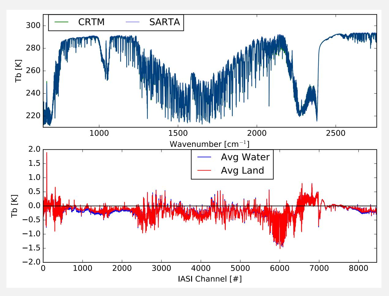
Comparison of CRTM and SARTA over land and ocean for the IASI instrument. The MISTIC instrument covers the spectrum range from 1734.70 cm-1 to 2449.18 cm-1 (590 channels).
