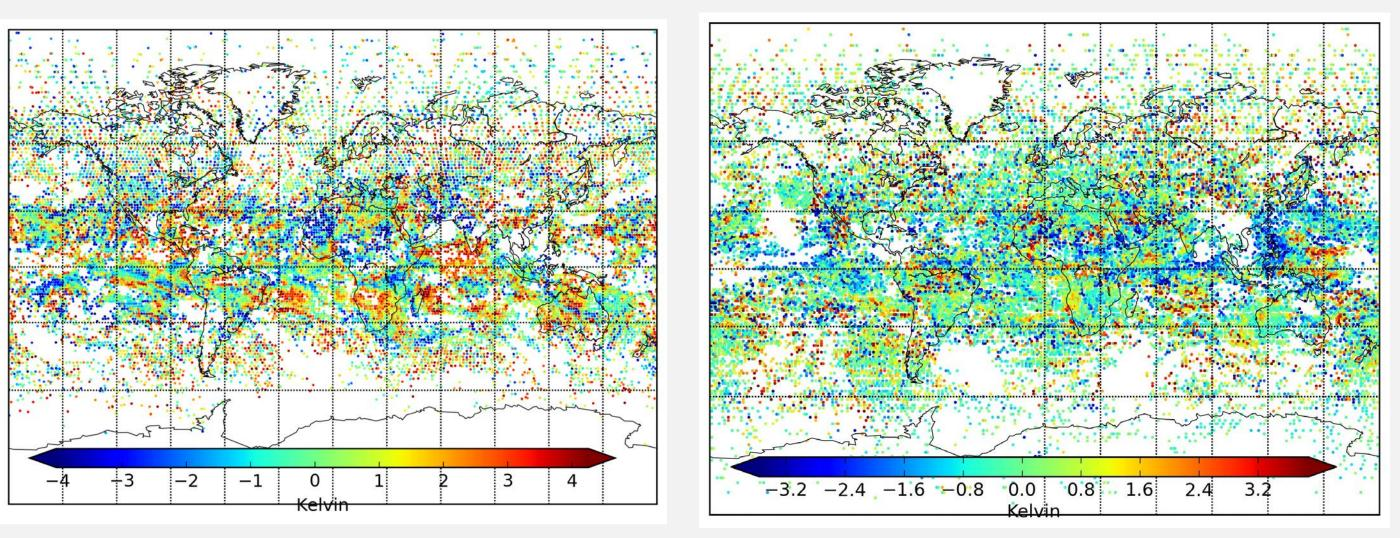
Observation minus forecast (OMF) for the MISTIC observations (Chan. 1839.15 cm<sup>-1</sup>) assimilated using the GMAO GEOS-5 data assimilation system. Left panel is for the real and right for the synthetic OSSE observations.
