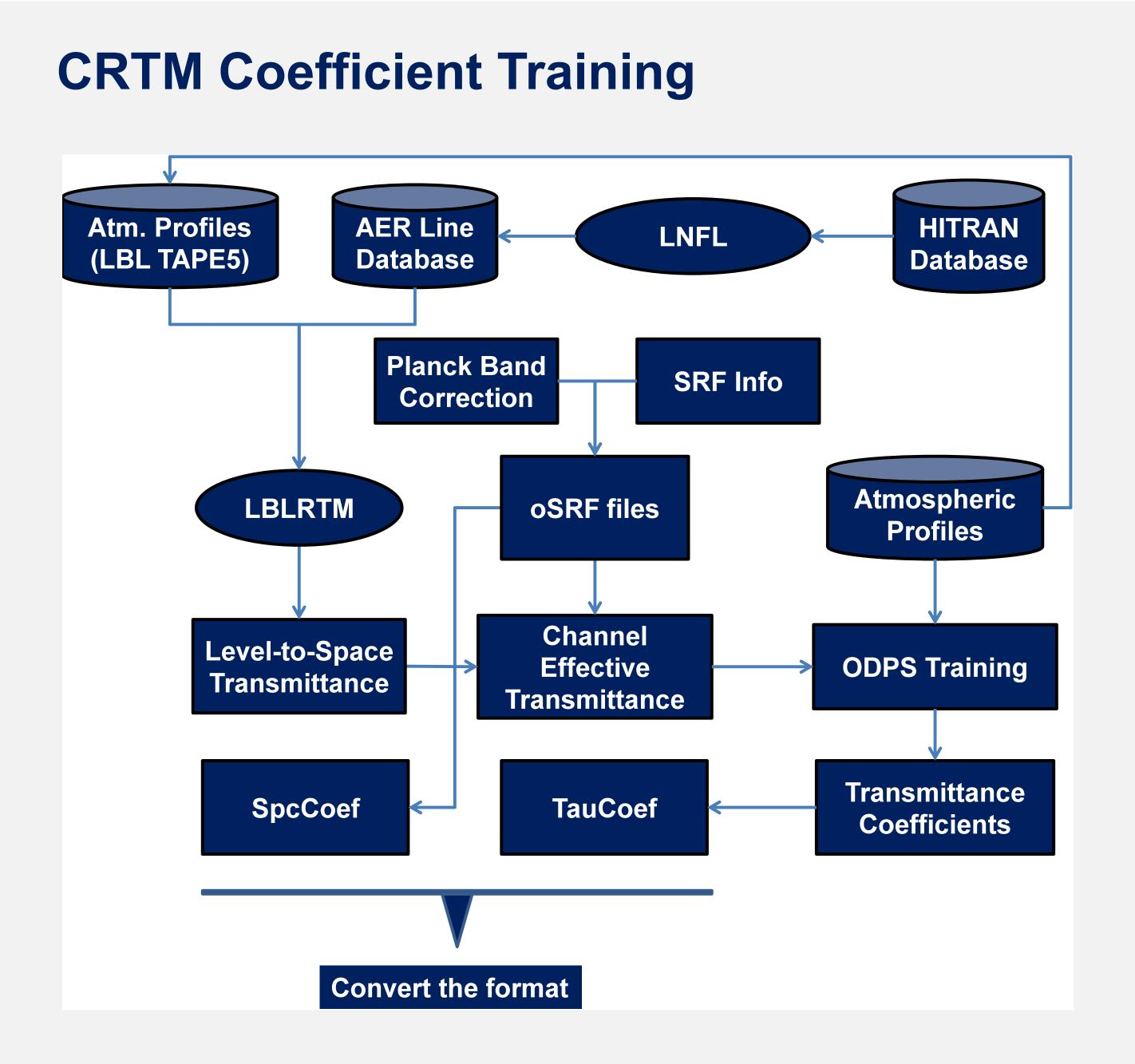
The CRTM Training process includes four major steps: (i) generating the SpcCoef files which include the sensor specific information, e.g., frequency of the channels, (ii) calculating the absorption coefficients using a line-by-line model, (iii) convolution of the absorption coefficients and the sensor response function, and (iv) regressing the sensor absorption coefficients vs. geophysical variables such as water vapor, ozone, temperature, and/or a combination of them.
