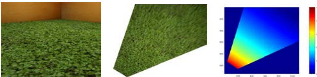
Fig. 4. Left: input image of a floor plane (green texture). Center: rectified image of the plane. Right: confidence map C for the rectified image, the Jet colormap (high values in red and low values in blue) shows that the value of trust decreases for the pixels that have a lower quality, i.e. those on the top right part of the image.
