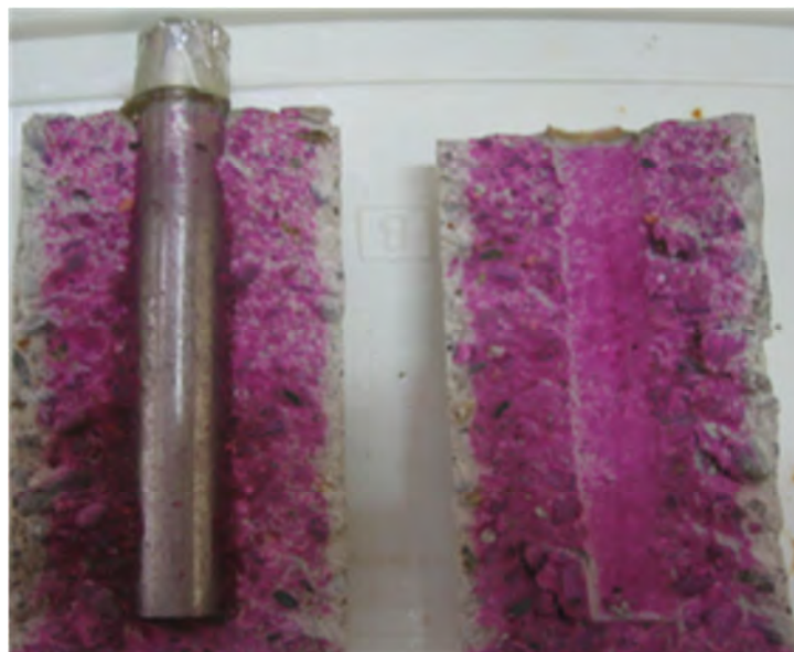
Figure 2-7 Non- carbonated sample; phenolphthalein test gives a pink color due to higher pH values. Steel bar has a shining surface and no corrosion products.
