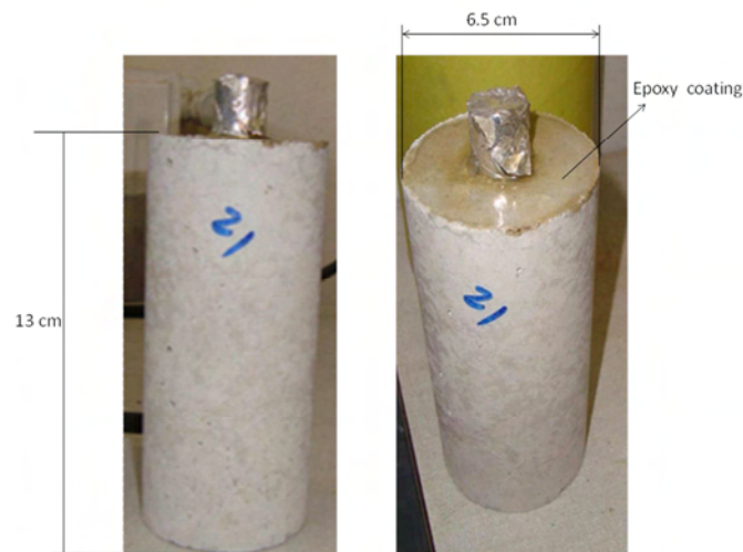
Figure 2-4 Final shape and size of lollypop samples
