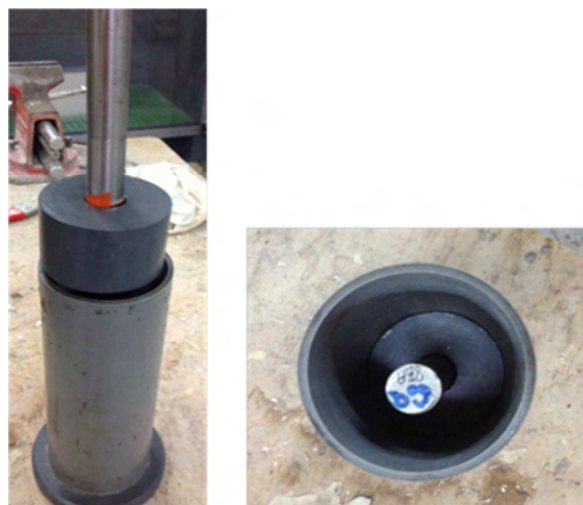
Figure 2-3 Sample preparation before pouring of concrete
