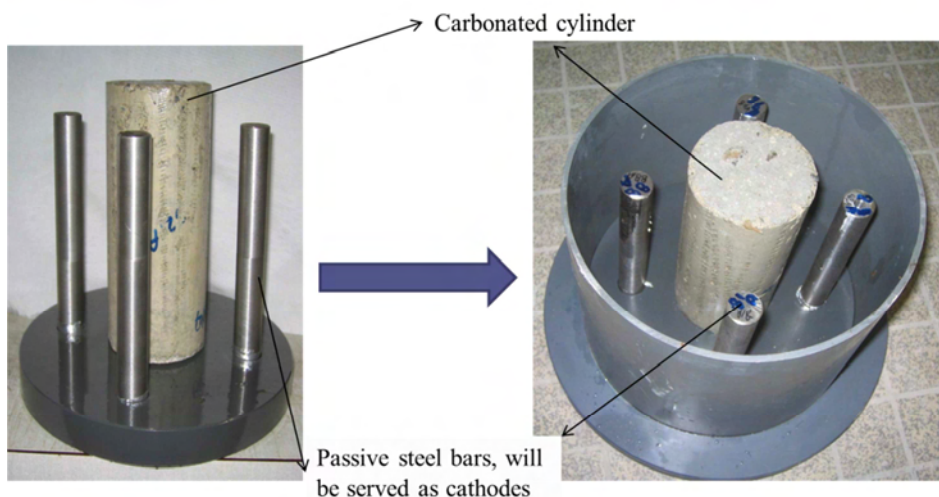
Figure 3-2 Fixation of carbonated inner cylinder and passive steel bars into the base plate and then in the mould.
