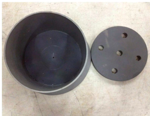
Figure 3-1 The preparation of specimen for accelerated corrosion tests, used mould with all the dimensions. (Dimensions are in cm).
