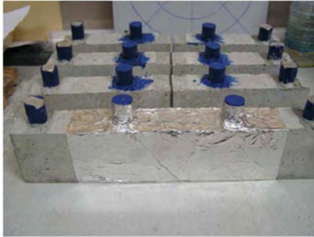
Figure 1-25 Galvanic samples with active and passive bars (Fortuné, 2009)
