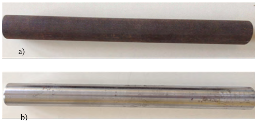
Figure 2-2 a) Steel bar before treatment, oxide layer is covering the steel surface b) Steel bar after mechanical treatment of brushing
