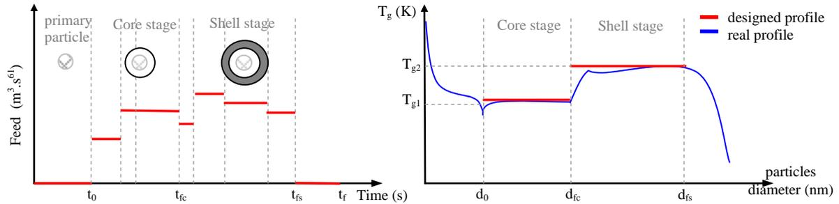
Fig. 1: Optimal feed rates and resulting glass transition temperature profiles
