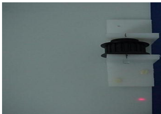
Figure 6.8: The pulleys on the other end of the timing belt held with two angular parts.
