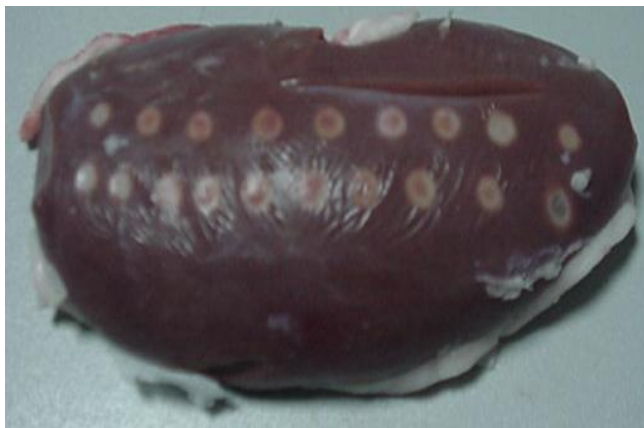
Figure 10.3: Lesions created in pig kidney demonstrating the excellent repeatability of the positioning device.
