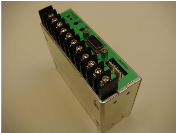
Figure 5.7: A photo of dedicated driver for Shinsei USB60 series, Shinsei D6060E.
