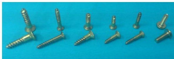
Figure 6.4: The brass screws used to mount the parts of the positioning device.
