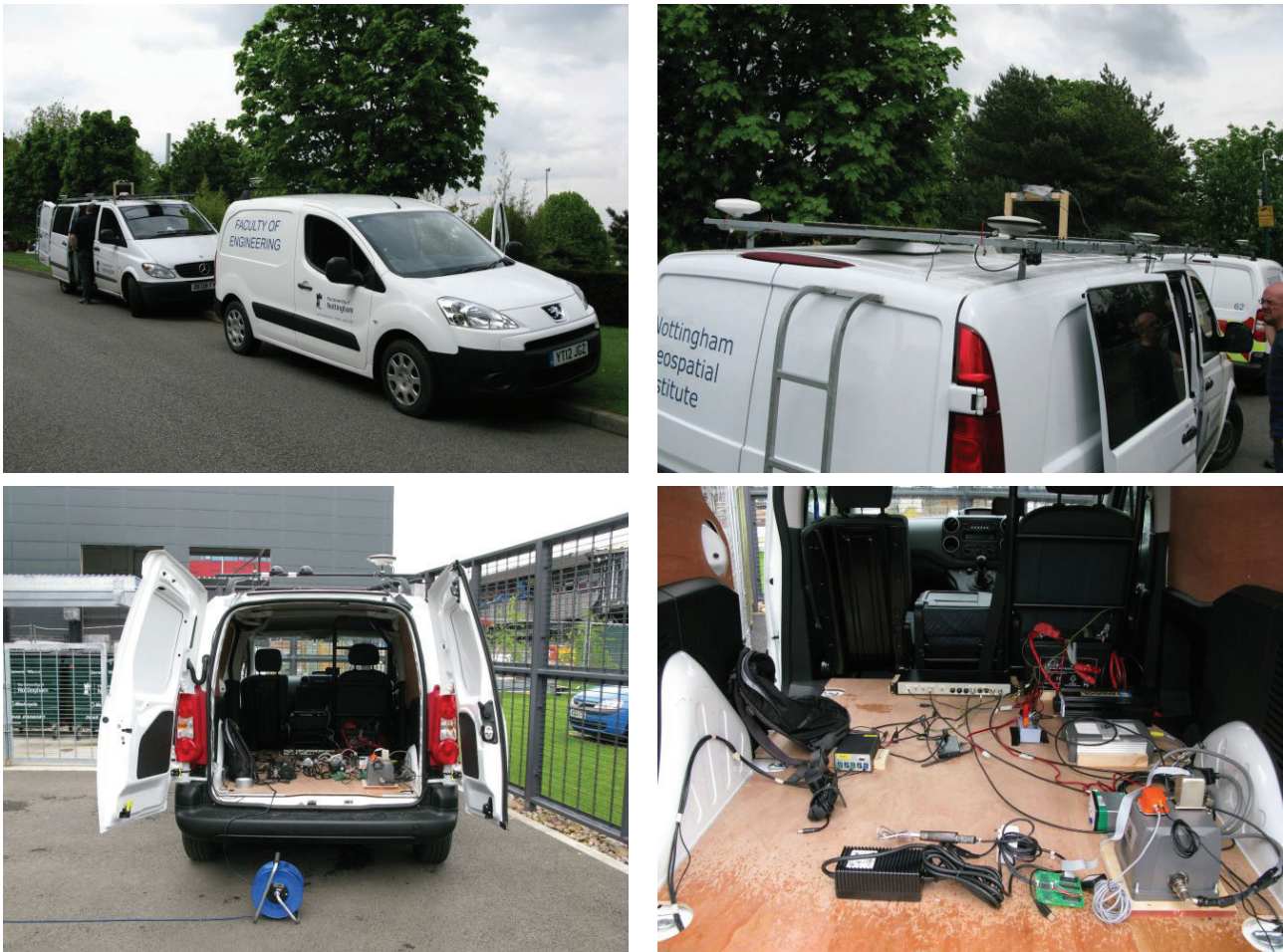
Figure 11: Two mobile mapping vans equipped with GNSS receivers, inertial sensors and DSRC transceivers.
