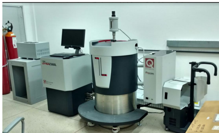
Figura 3.12: Magnetômetro PPMS ( physical property measurement system ) DynaCool da marca Quantum Designs do GNMS-UFRN usado para as medidas magnéticas.
